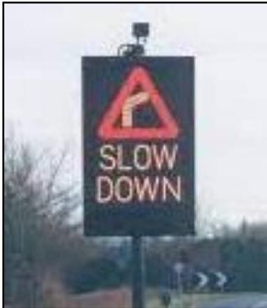
This is a VAS (Vehicle activate sign). In this example the sign is also activate by the speed of a vehicle but rather than presenting feedback to the driver it illuminates (when triggered) a standard traffic sign to warn the driver of an upcoming hazard
