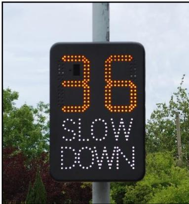
This is a typical SpID device. As a vehicle approaches the sign it checks the speed and if required illuminates a message which can include a speed, happy/sad face, safety message etc.
